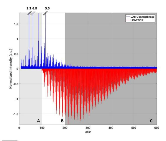
Figure 2: Comparison of positive ions mass spectra (1) LAb-CosmOrbitrap, in blue, top panel and (2) LDI-FTICR, in red, lower panel in reverse scale. Intensities of three peaks (m/z 43.0290; 60.0556 and 114.9033) in the LAb-CosmOrbitrap mass spectrum are out of the window and thus reported at the top the window. Mass spectra are separated in three distinct zones named A, B and C. Each zone is detailed in a specific result section.
