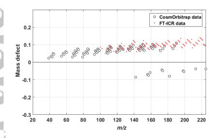
Figure 4: Mass Defect versus Exact Mass diagram (MDvEM) derived from mass spectra presented in Figure 1. Red dots represent ions from the LDI-FTICR mass spectrum. Black open circles represent ions from LAb-CosmOrbitrap mass spectrum.
