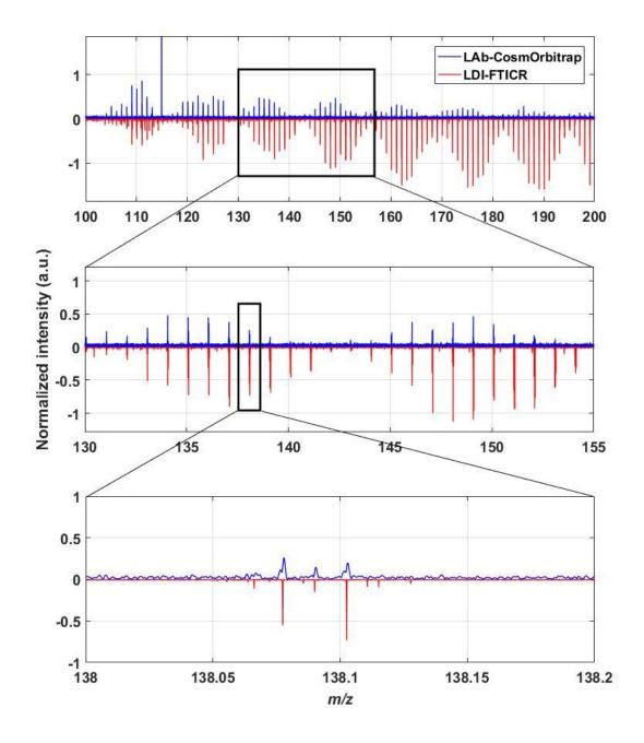
Figure 3: Focus on three distinct zones in the LAb-CosmOrbitrap and LDI-FTICR mass spectra, as presented in Figure 1. The first window (top) shows m/z from 100 to 200. A black box indicates the next window (middle) from m/z 130 to 155. Again, another black box indicates the last window (bottom) from m/z 138 to 138.2. As a reminder from the Figure 1, the LAb-CosmOrbitrap mass spectrum is the blue top panel and the LDI-FTICR mass spectrum the red low panel in reverse scale.
