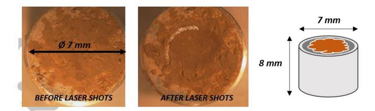
Figure 1 : Pictures of the Titan's tholins powder pressed onto the indium sample-holder of the LAb-CosmOrbitrap before laser shot (left) and after laser shots (middle). On the middle picture, laser shots are visible on the brown tholins powder, demonstrating the ablation of the sample. The scheme (right) illustrates dimensions of the sample-holder (8 mm height and 7 mm diameter).
