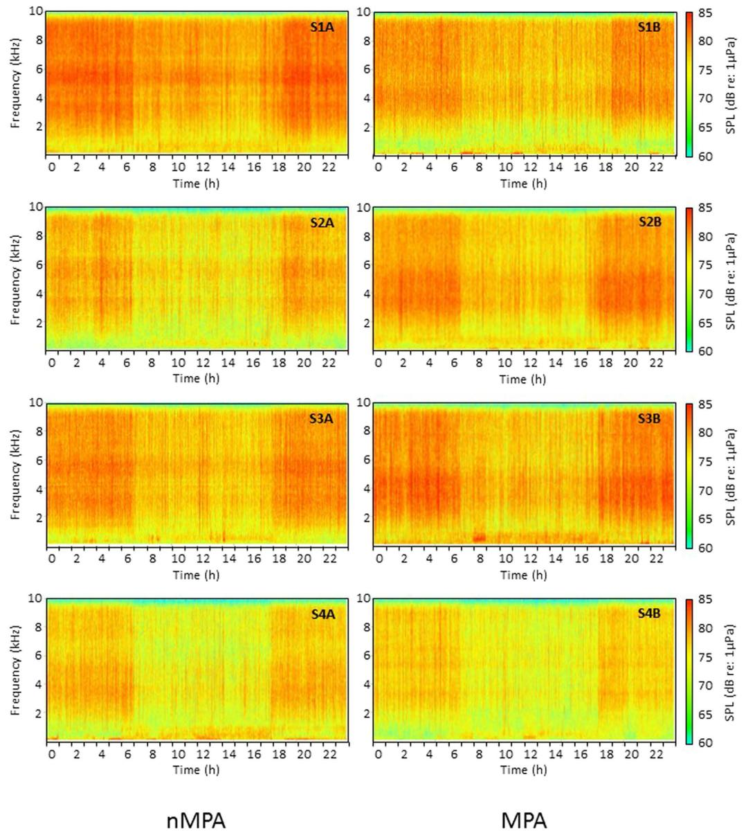
**Figure 2.** Spectrograms showing examples of 24 h of data from each recording sites. Spectrograms were obtained by concatenating 1s sound samples per hour during the first 24h of the first replicate (FFT size 512 points, Hamming window).
